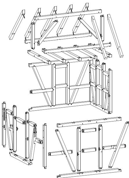
To assemble the roof, lay down the ceiling beams and join the king posts with the knee braces and the ridge pole. Now attach the plates and the king posts to the ceiling beams and secure them with wooden pegs.
